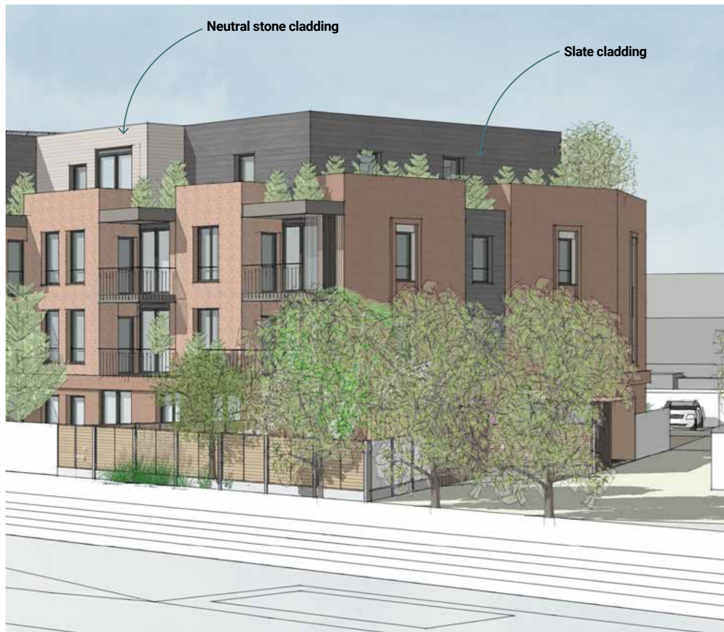
Proposed north elevation and upper level materials
